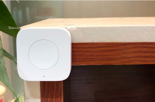
In response to the call for energy conservation and emission reduction, Jinmao Zhuhai has installed intelligent switches, human sensors and other devices in the office area to enable switching off at regular times and remote control of lights as well as automatic switching of lights when no movement is detected in 30 minutes and wall-mounted air conditioners with a view to reducing waste of resources
